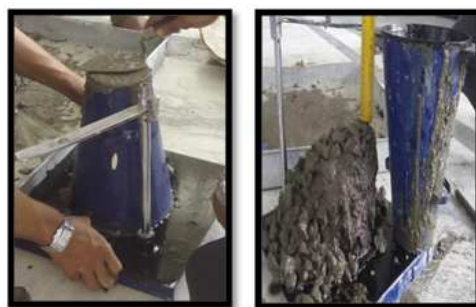
Figure 3.1: Slump Test for Fresh Concrete
