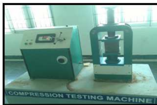
Figure 4.1: Compression Test for Concrete Cubes
