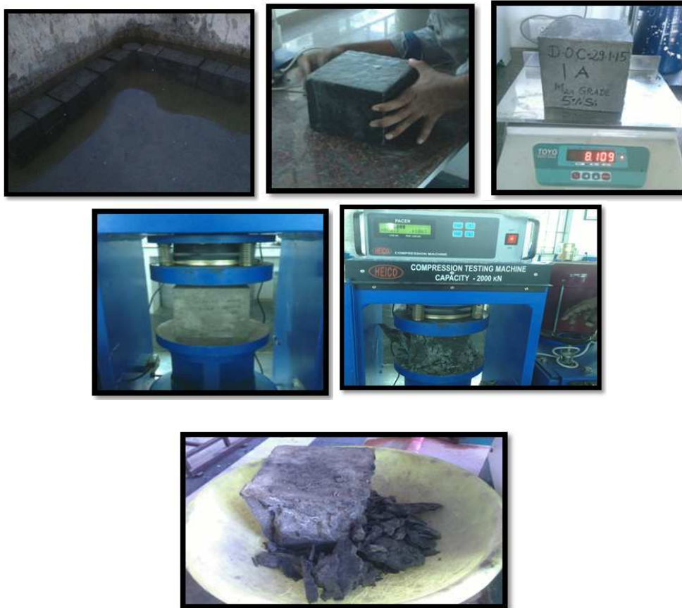
Figure 4.2: Cube Curing and Testing
