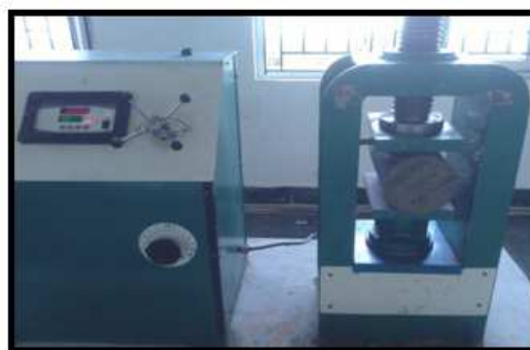
Figure 4.3: Split Tensile Test for Concrete Cylinder
